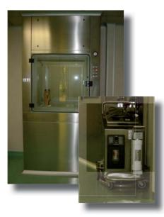
The **Pass Box** works to transfer the material between areas with different cleanliness grade. The materials may cross the Pass Box in both directions by different handling operations through two interlocked doors. A double inlet centrifugal motorblower provides a vertical airflow in the pass-trough chamber with two interlocked doors.
